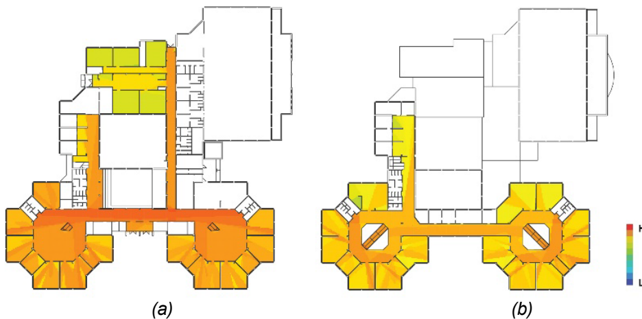
Figure 4. Visibility Graph Analysis – Visual Mean Depth red – integration, blue – segregation (more redness means less visual mean depth)
